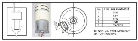
5). If you need the speed adjustable and controllable function, then wire as this.
